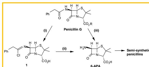
Figure 3. Synthesis of 6-aminopenicillanic acid catalyzed by immobilized penicillin G amide [32].
